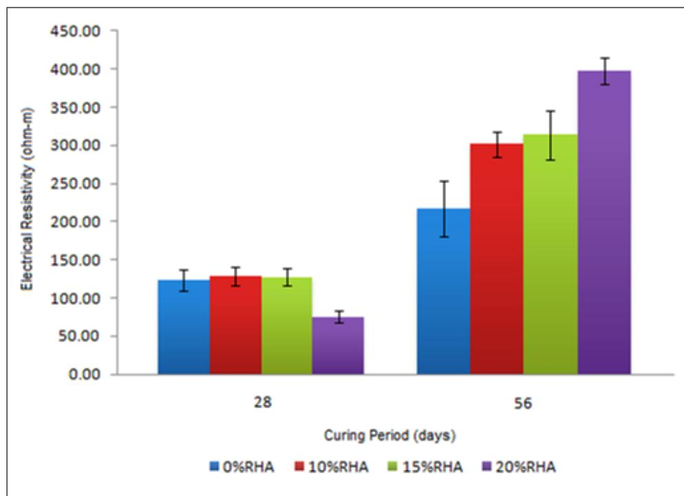
**Figure 6.** Electrical resistivity of RHA concrete cured for 28 and 56 days
