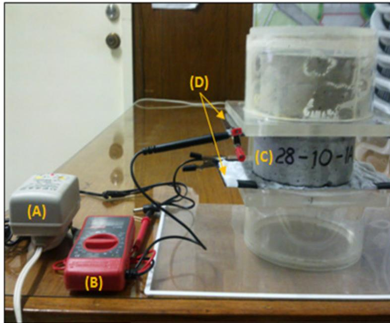
**Figure 5.** Test set-up for DC electrical resistivity determination, where, (A) DC Power Supply, (B) Digital Multimeter, (C) Concrete Test Specimen, and (D) Stainless Steel Plates.
