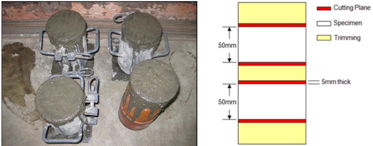
**Figure 4.** Parent concrete specimens cast in 100 x 200mm molds (left) with the schematic diagram of the specimen cutting planes (right)
