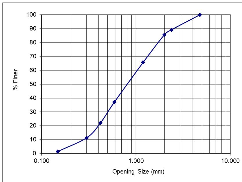
**Figure 3.** Particle size distribution of fine aggregates
